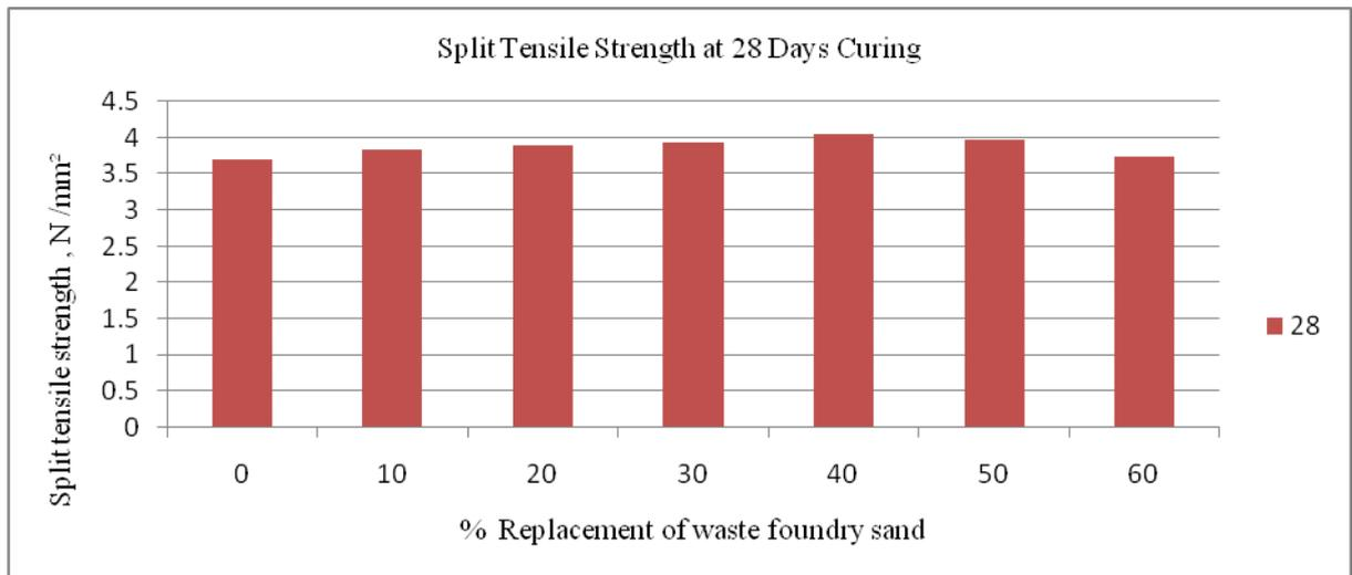
**Graph 4. Percentage Replacement of Waste Foundry Sand V/s Split Tensile Strength for 28 days**
