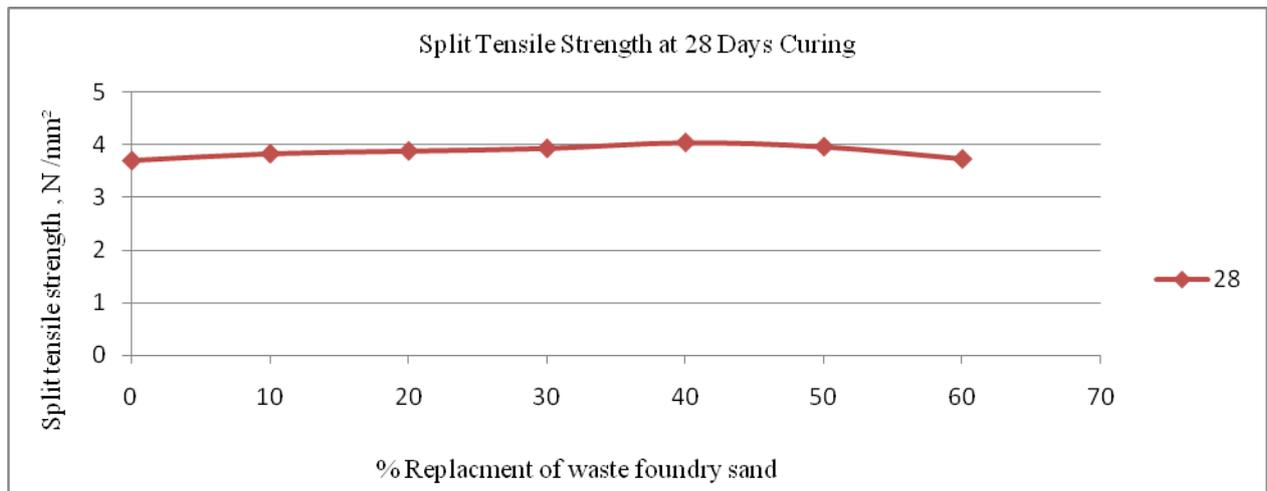
**Graph 5. Split Tensile Strength of Various Concrete Mixes with Replacement of Fine Aggregate over Waste Foundry Sand at 28 days.**
