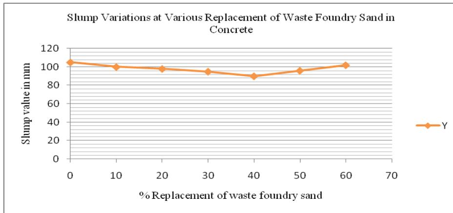
Graph 1. Slump Variation at Various Replacement of Waste Foundry Sand in Concrete
