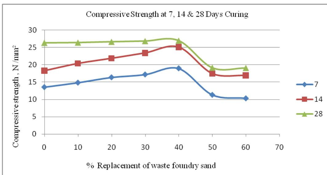
Graph 3. Compressive Strength of Various Concrete Mixes with Replacement of Fine Aggregate over Waste Foundry Sand at for 7, 14, 28 days.
