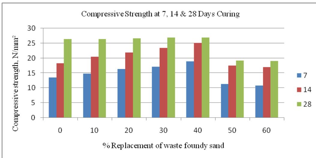
Graph 2. Percentage Replacement of Waste Foundry Sand V/s Compressive Strength for 7, 14, 28 days.
