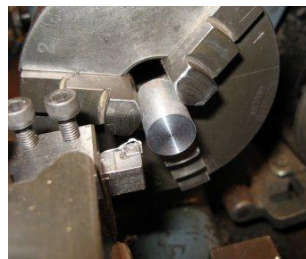
Fig. 3 Conventional Turning Setup
