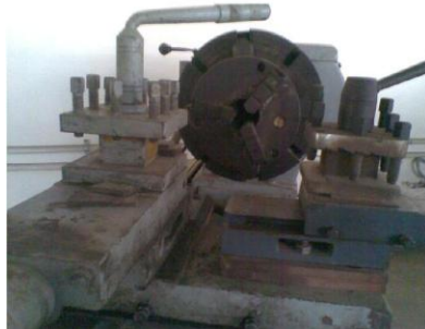
Fig. 5 Multi Tool Turning Setup
