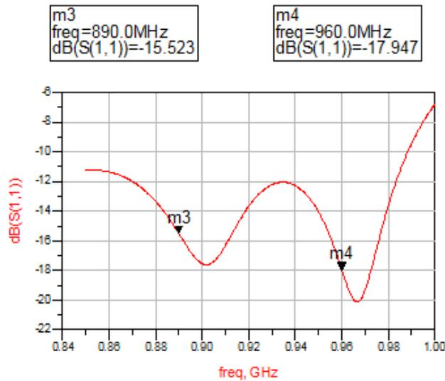
**Figure9. Return loss of the duplexer**
