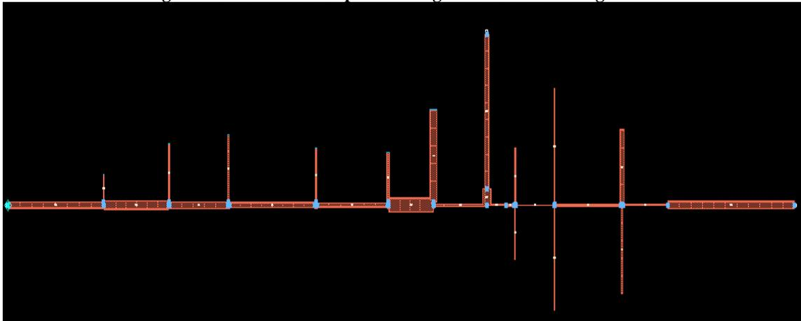
Figure7. Layout of duplexer using filters and matching circuit
