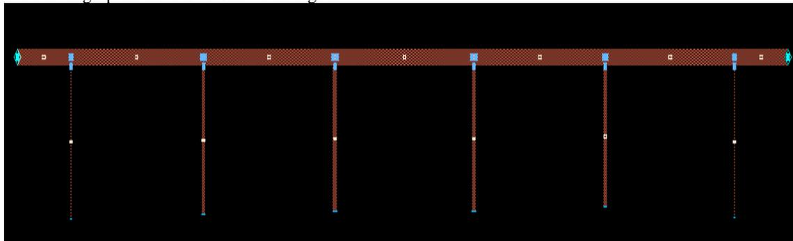
**Figure 4. Layout of microstrip highpass filter**
