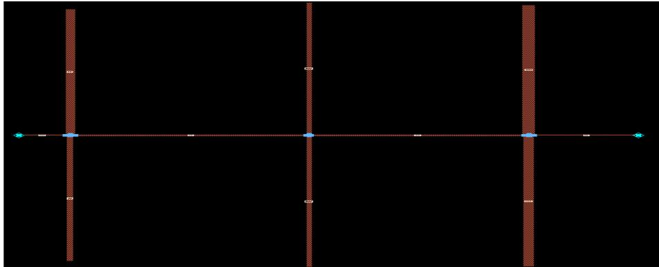
Figure2. Layout of microstrip lowpass filter
