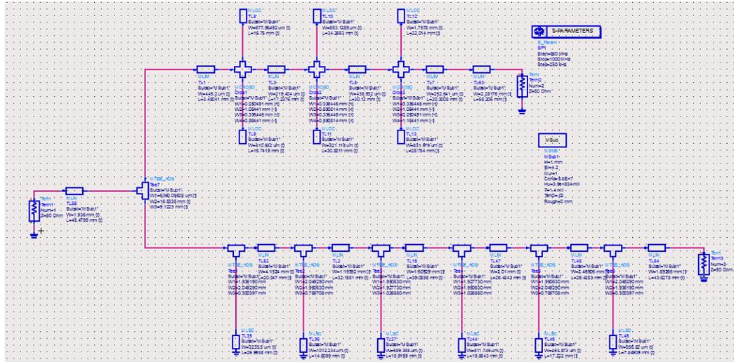
Figure6. Schematic of duplexer using filters and matching circuit
