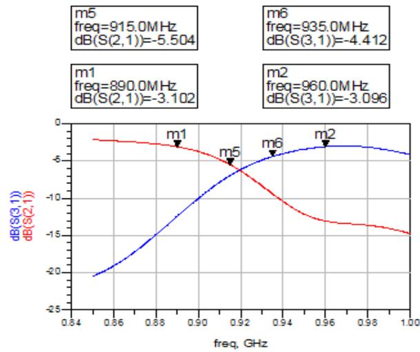
**Figure8. Transmission loss of the duplexer**
