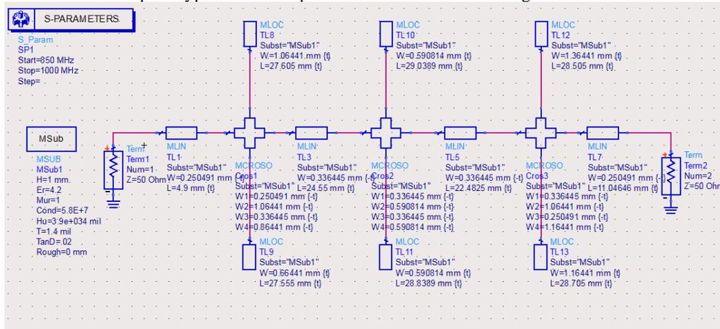
**Figure1. Schematic of microstrip lowpass filter**
