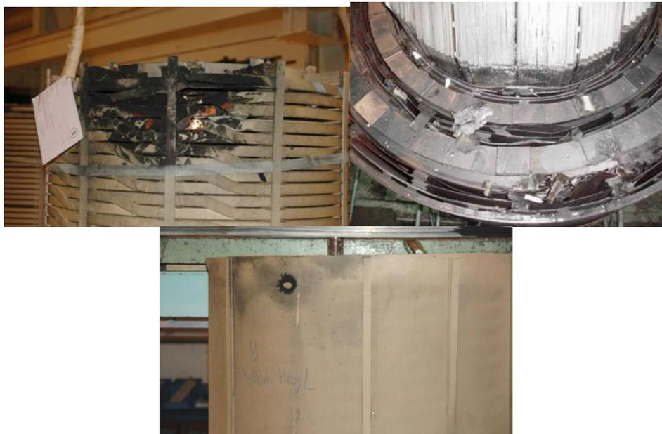
*Figure 5. Problem in core and winding*
