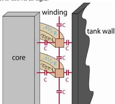
Figure 2. The simplified network behavior of a transformer's active part
