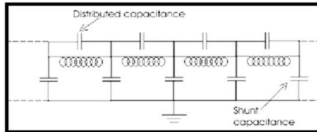
**Figure 3. Distributed RLC network of transformer**
