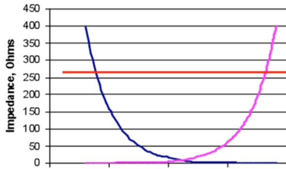
Figure 1. Impedance of an ideal resistor, capacitor and inductor
