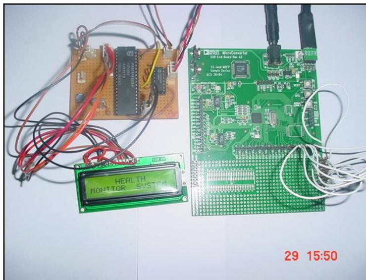
**Fig.3 – Communication set-up for the Health Monitoring System**
