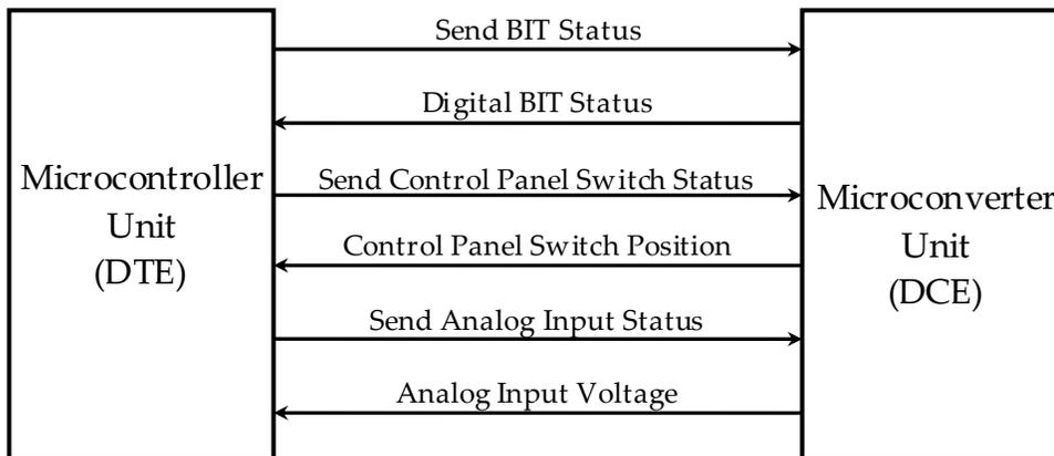
**Fig.2 – Serial Communication between DTE and DCE**
