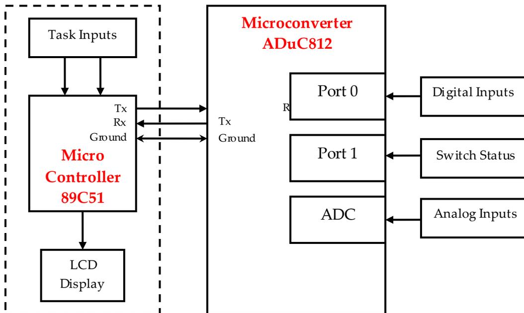
**Fig. – 1 Block Diagram of the Proposed Scheme**
