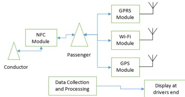
Fig 1: Block Diagram of Modules Used in SmartBus
