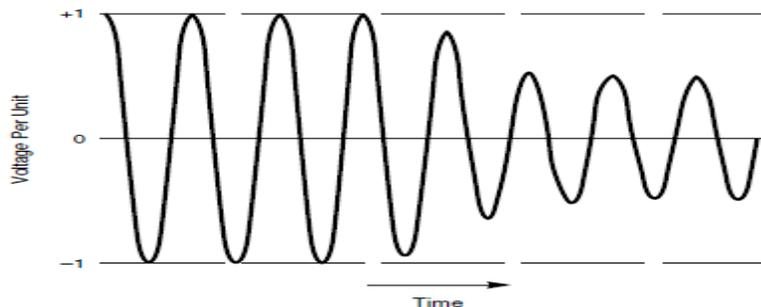
Fig.5.Under voltage plot
