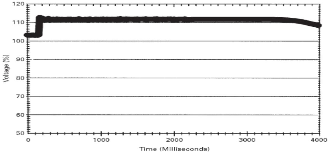
Fig.4.Long duration overvoltage plot
