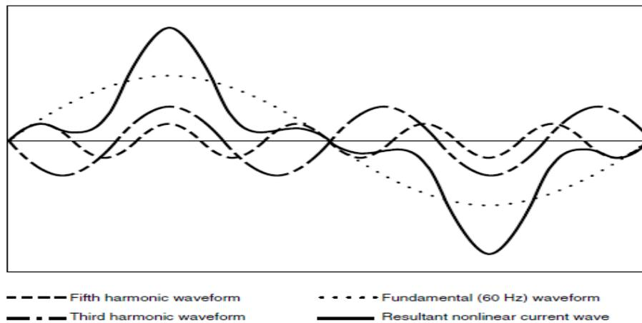
**Fig.8. Composite harmonic waveform.**
