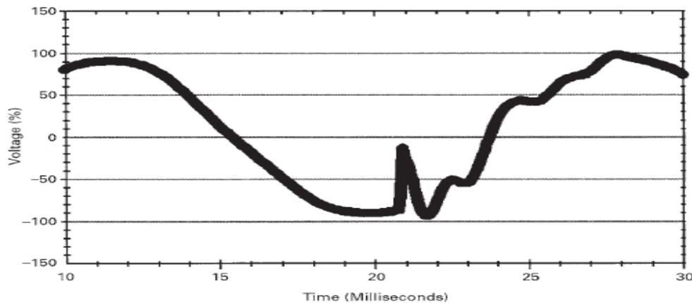
**Fig.7. Impulsive transient plot.**
