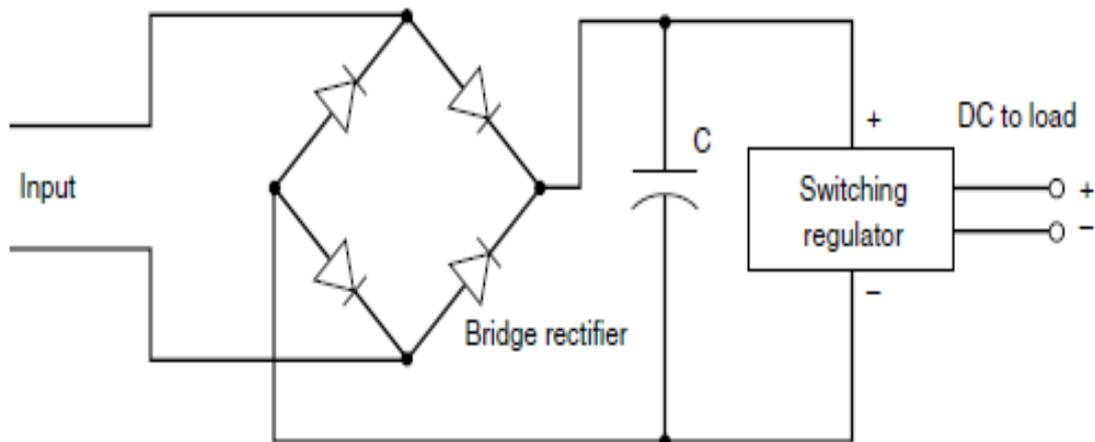
*Fig.10. Switch mode power supply*
