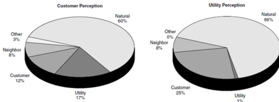
**Fig. 1. Results of a survey on the causes of power quality problems. (Courtesy of Georgia Power Co.)**
