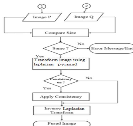
Fig.4 Flowchart of the proposed fusion process
