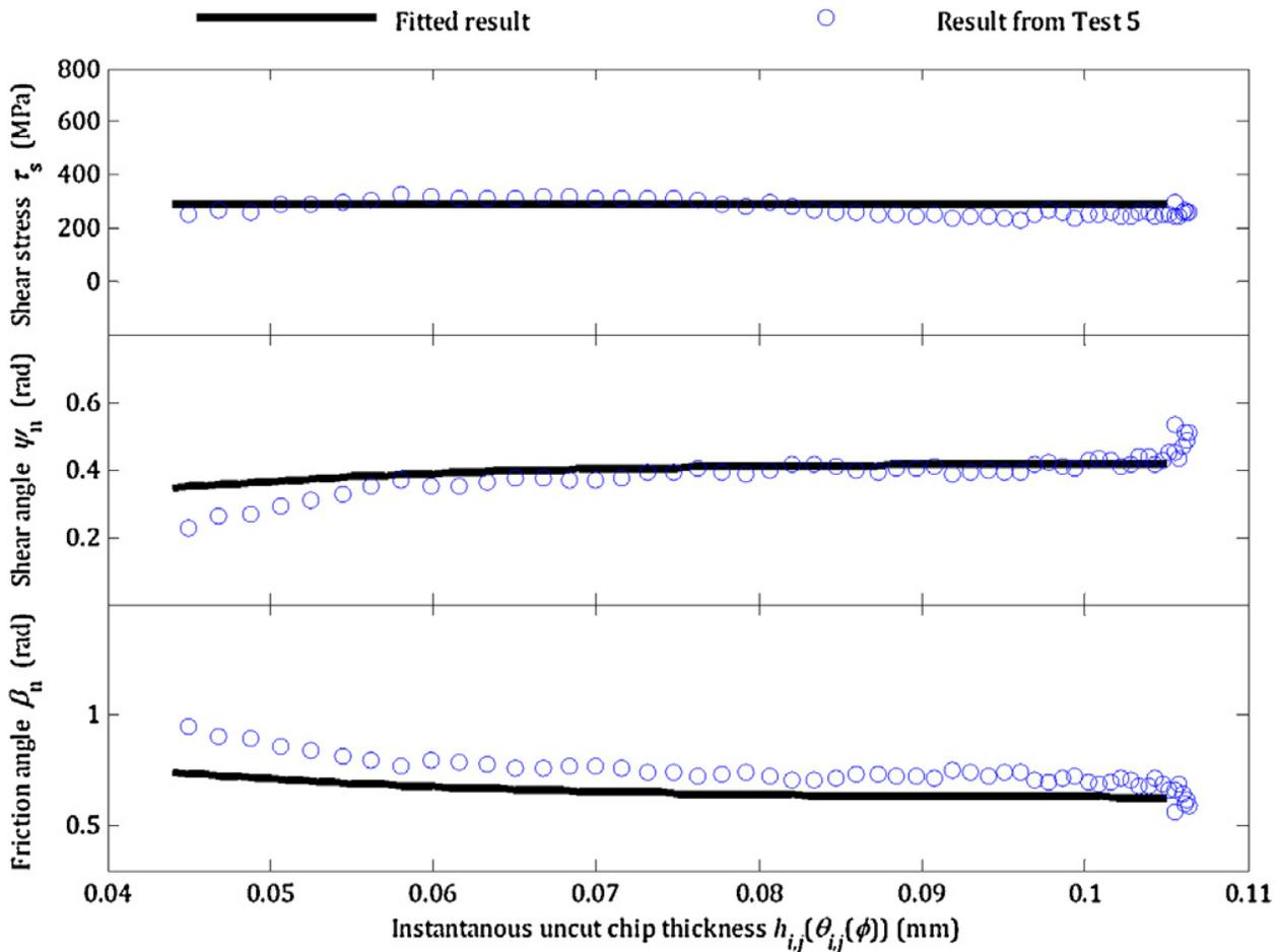
**Fig.3.1** Comparison of uncut chip thickness Vs  $\beta_n, \tau_s, \psi_n$
