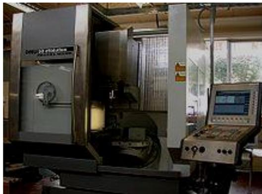
**Fig.7** Five-axis machining center with rotating table and computer interface
