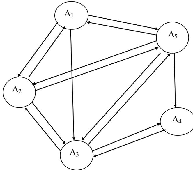
**Fig. 1** Digraph representing interdependence among factors 1 work material 2 cutter runout, 3 tool geometry, 4 penetration strategies, 5 machine tool
